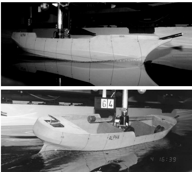
Figure 3. Tenacious model during heeled and yawed tests
