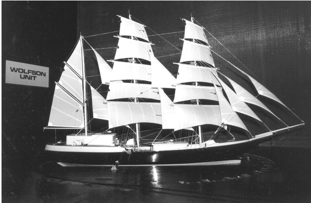
Figure 4. Wind tunnel model with full sail set
