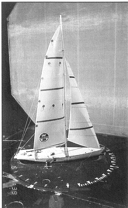
Fig 4. A model monohull yacht in the wind tunnel for gust heeling tests by the Wolfson Unit.
