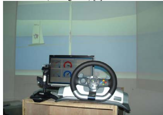
Figure 2. Advanced Display Environment showing wheel and curved display panels for VR driven by 3 data projectors [8].
