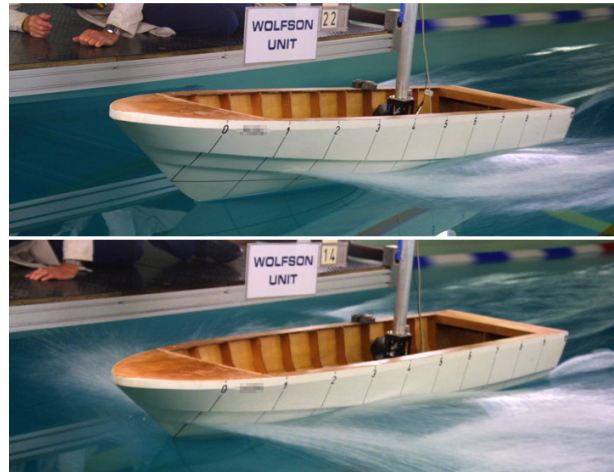
Fig.6 - tests at 30Kn, different interceptor depths: no interceptors fitted (top), 40mm interceptors fitted (bottom)
