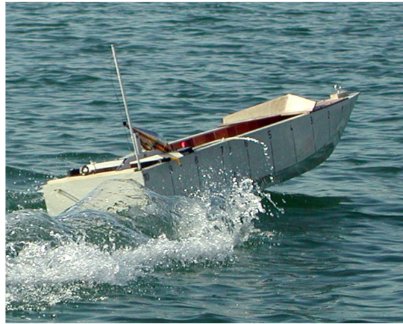
Fig.2 – Manoeuvring tests on a model Patrol Boat for Colombo Dockyard Ltd.
