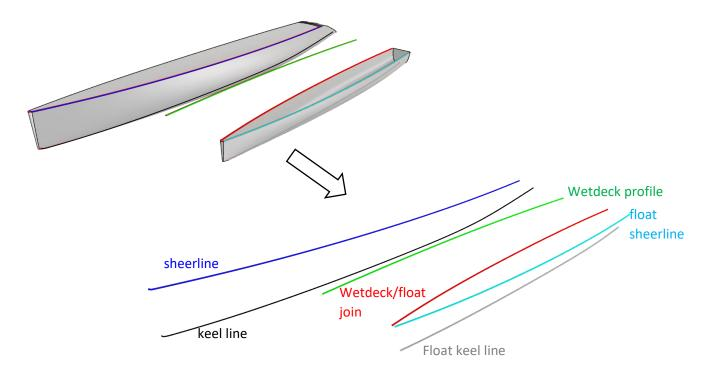
Therefore in the case of a trimaran, the wetdeck width (and between hull distance) is the distance between the main hull sheerline curve and the wetdeck/hull join curve. The wetdeck profile curve is still used to determine the extents and height of the wetdeck.
