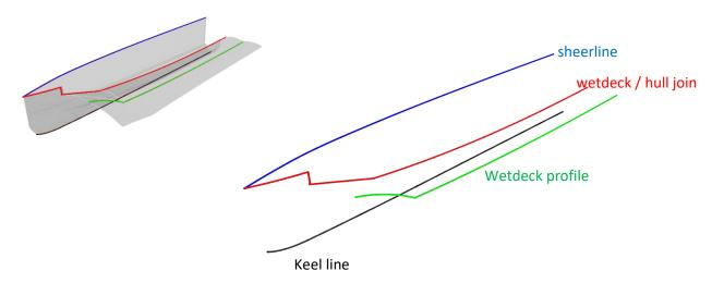
The approach taken within Hullscant has been to allow for 2 more sets of station curves, from which these lines can be taken.
