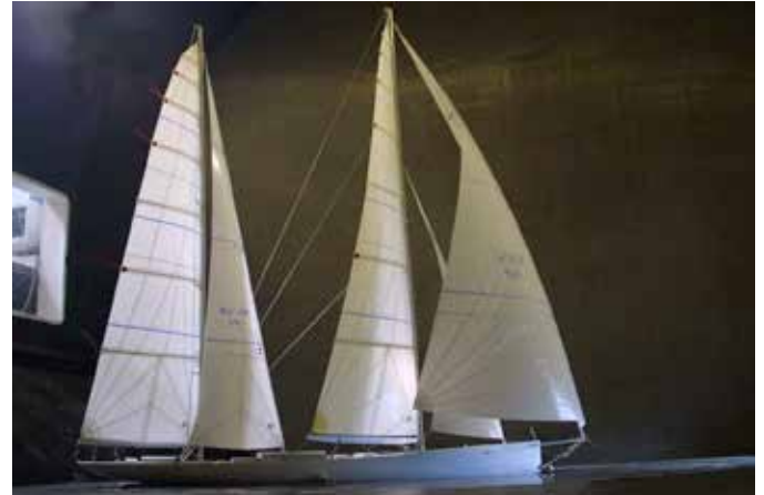
Wind tunnel sail development for '67m Hetarios Ketch' - Dykstra Naval Architects
